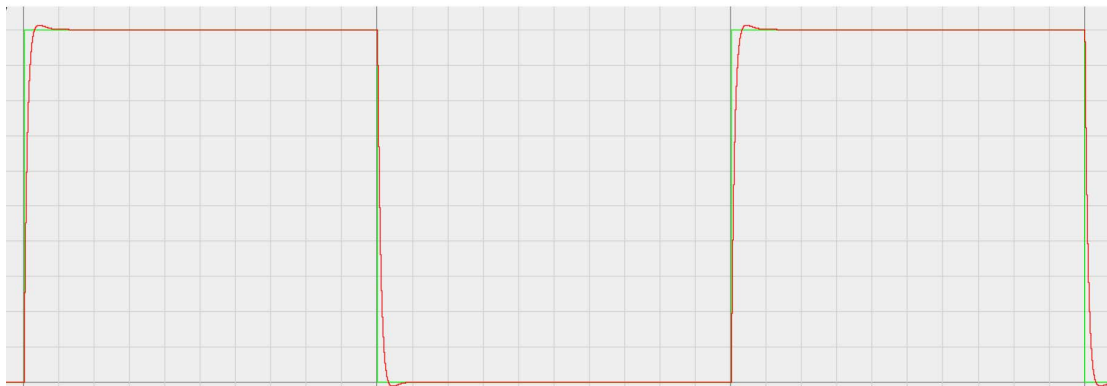
Fig. 5 PI control system with the zero at -12. (Photo/Picture credit: Original)
