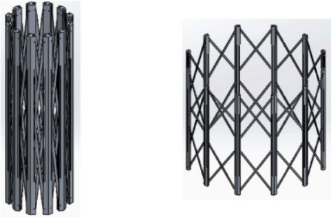
Fig. 6 Truss inside antenna [8].
