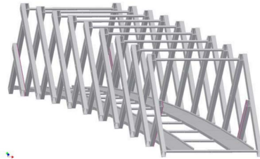
Fig. 3 Conceptual diagram of the development of a foldable bridge by Hiroshima [6].
