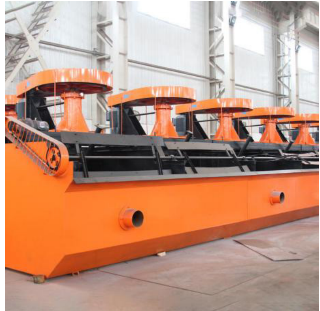
Fig. 2 The SF series flotation machine, manufactured by Luoyang Zhongde Heavy Industries Co., Ltd [8].
