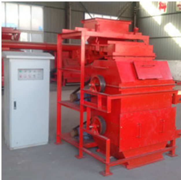
Fig. 1 The CXY.Q model high-intensity magnetic separator for titanium, nickel, and manganese, manufactured by Henan Strong Magnetic Separation Equipment Co., Ltd [7].
