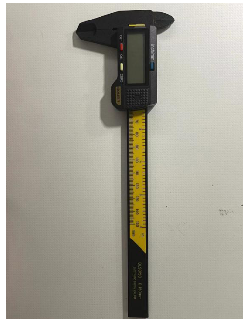
Figure 10 The digital display simple caliper The instruments for the experiments, including two mul-
