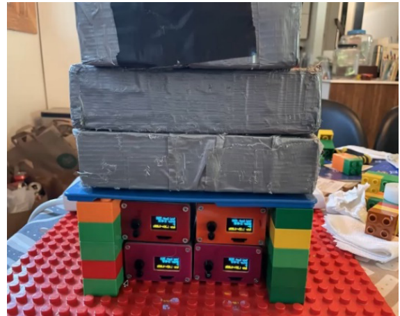
Fig.1. Left: How detectors 1 to 4 were placed. Brown rectangles are the detectors, the blue part placed on top of the detectors is the stand for lead, gray part is the lead added above the detectors. Right: Picture of how the detectors were built up.
